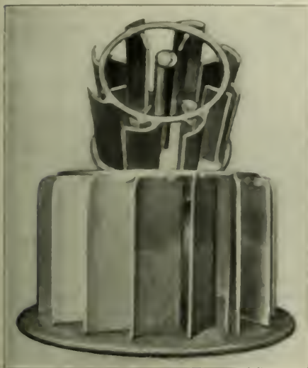
FIG. 3 ARRANGEMENT OF BLADING SHOWN IN SMALL MODEL
